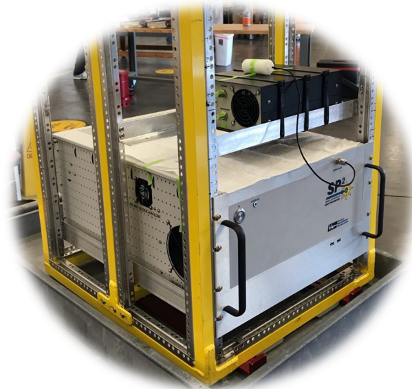
Figure 1: The Clemson University SP2 instrument preparing for field deployment on a research aircraft for measurements of black carbon aerosol from biomass burning and anthropogenic sources.
